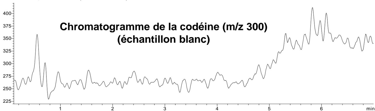
Ion chromatograms of the base peaks of  $[^2\text{H}_3]$ codeine (m/z 303) and codeine (m/z 300) (internal standard at 7.5 ng/mg) from 20 mg of extracted, drug-free, black human hair.
